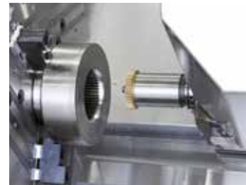
■ Shaping of gear teeth (Flanx-Spline)
