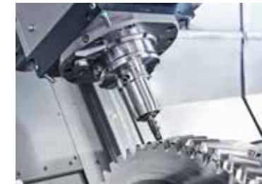
■ Milling of gear teeth (Flanx-LM)
