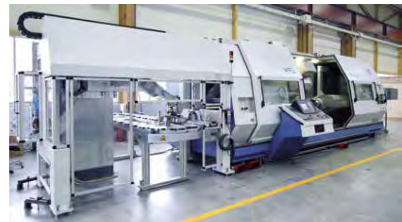
Gantry loader with rotary index magazine
