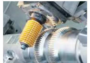
■ Hobbing of gear teeth (Flanx-Hob)
