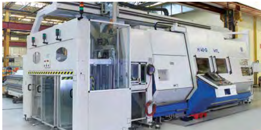
Gantry loader with loading hatch
