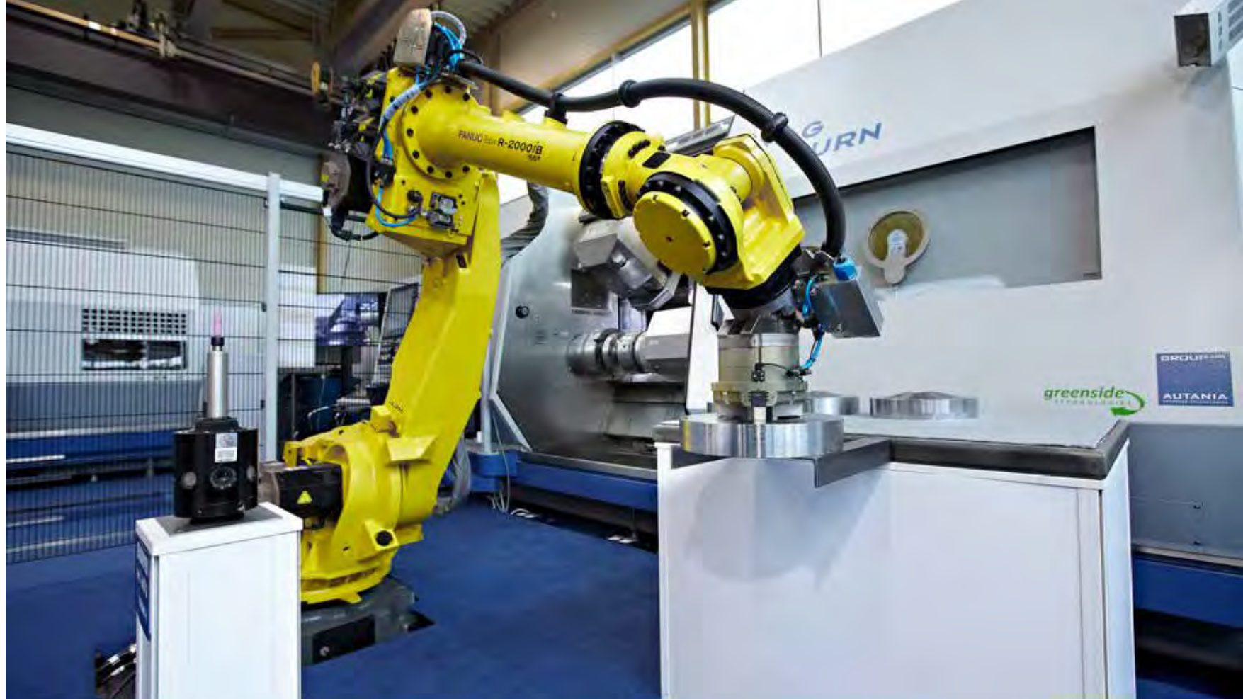
Buckling arm robot with deburring-station
