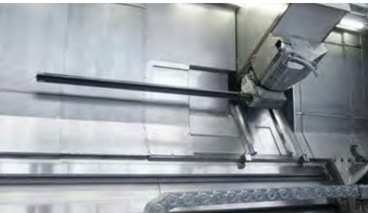
Deep hole drilling with automatic coolant docking
