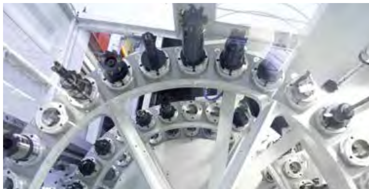
Maintenance-free disc magazine
