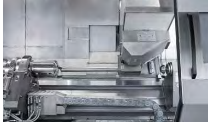
Internal machining with damped boring bar
