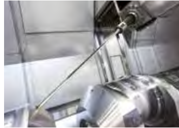
➤ Deep hole drilling
