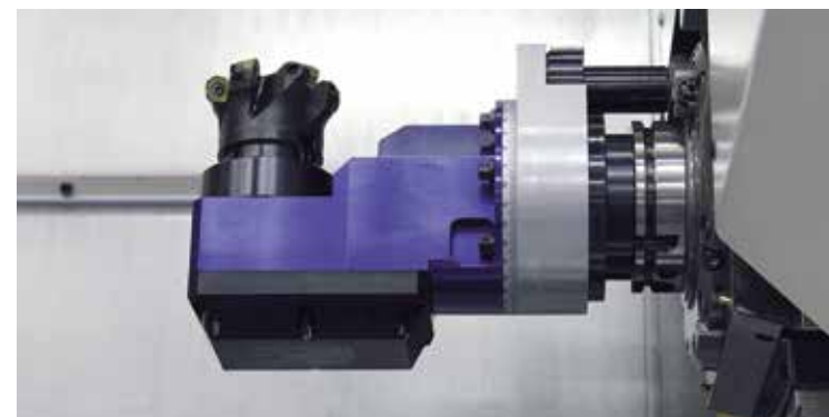
Angular head with torque support
