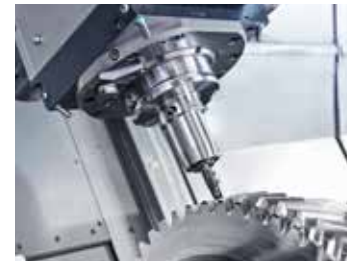
■ Milling of gear teeth (Flanx-LM)
