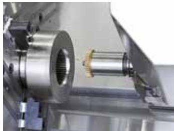
■ Shaping of gear teeth (Flanx-Spline)
