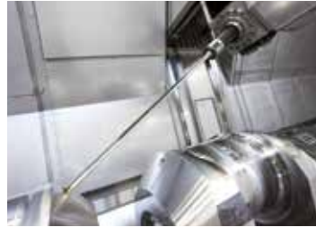
➤ Deep hole drilling
