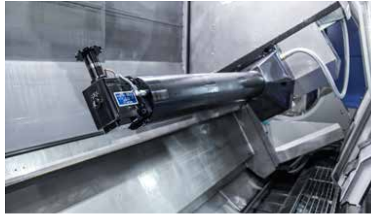
Internal milling with angular head
