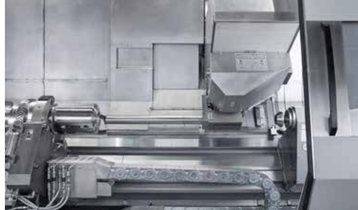
Internal machining with damped boring bar
