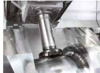
➤ Milling of crankshaft pins
