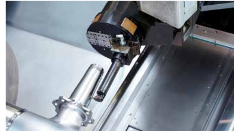
CNC facing head for complex spindle operations
