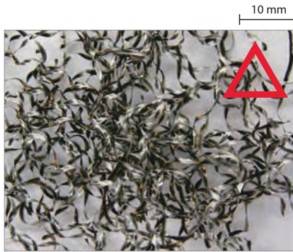
Without Chipbreaker (Conventional)
