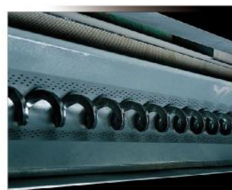
Automatic chip removal (Screw type chip conveyor)
