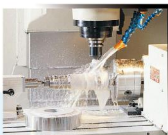
High pressure coolant (P:3.5 kg/cm 2 , Q:100 l/min)
